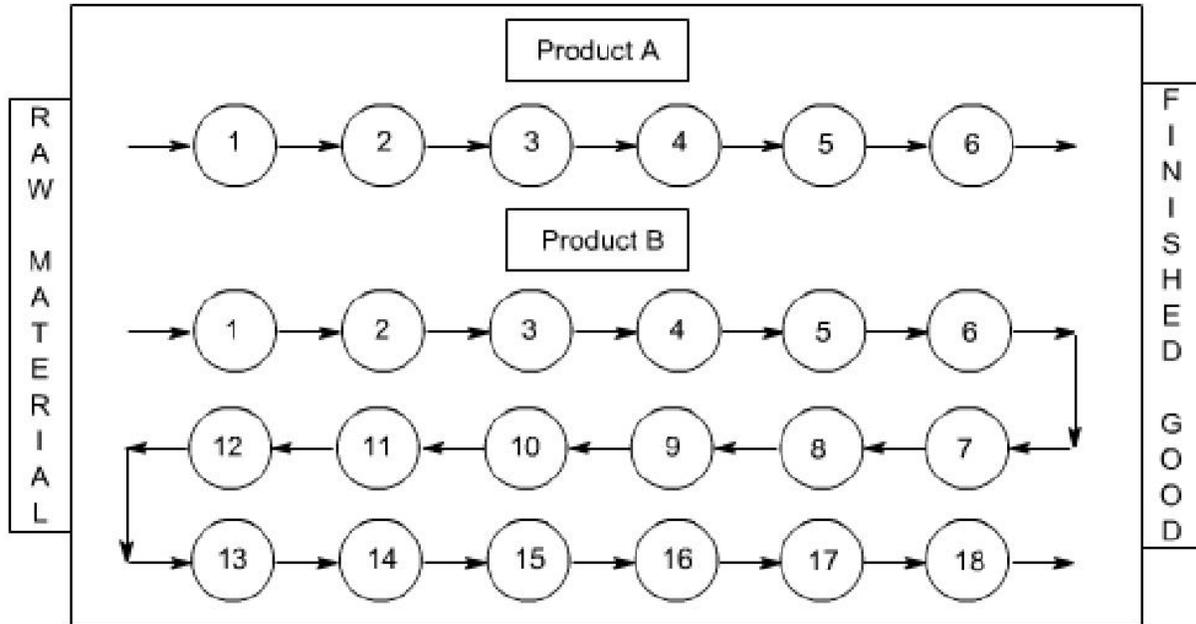
**Figure 2: A Pictorial Representation of Product Layout. Source (NPTEL).**
