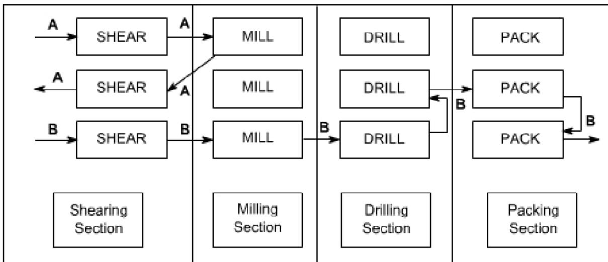
Figure 1: A Pictorial Representation of Process Layout. Source (NPTEL).
