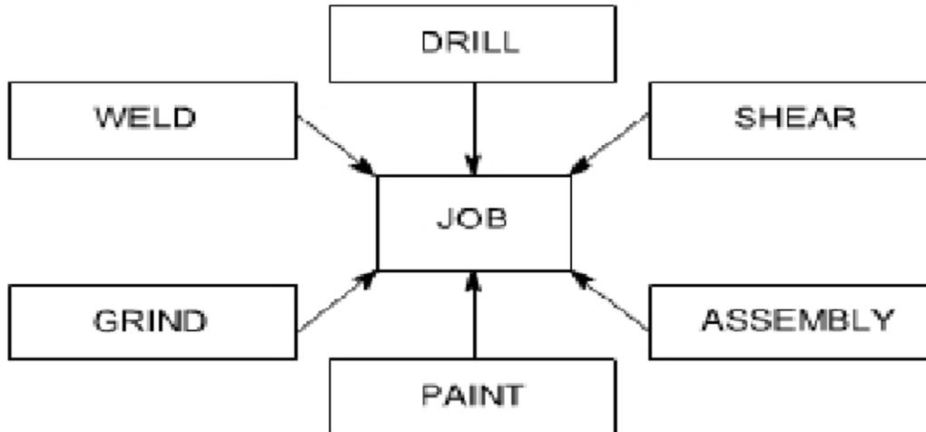
Figure 3: A Pictorial Representation of Fixed Position Layout. Source (NPTEL)
