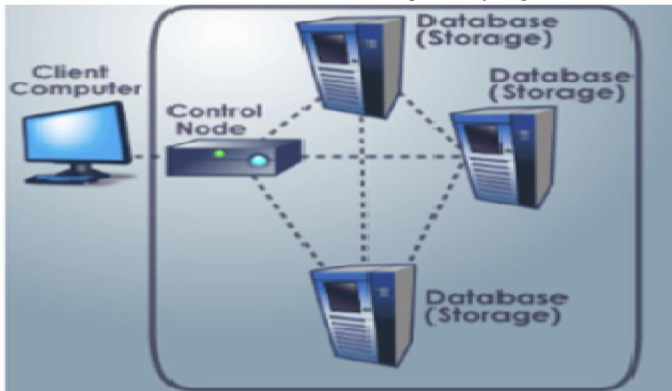
**Figure 3. A typical Cloud Storage system architecture**
