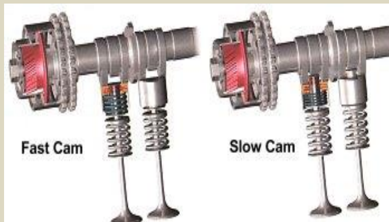
Fig. 5:-Vario-cam Plus uses hydraulic phasing actuator and variable tappets
