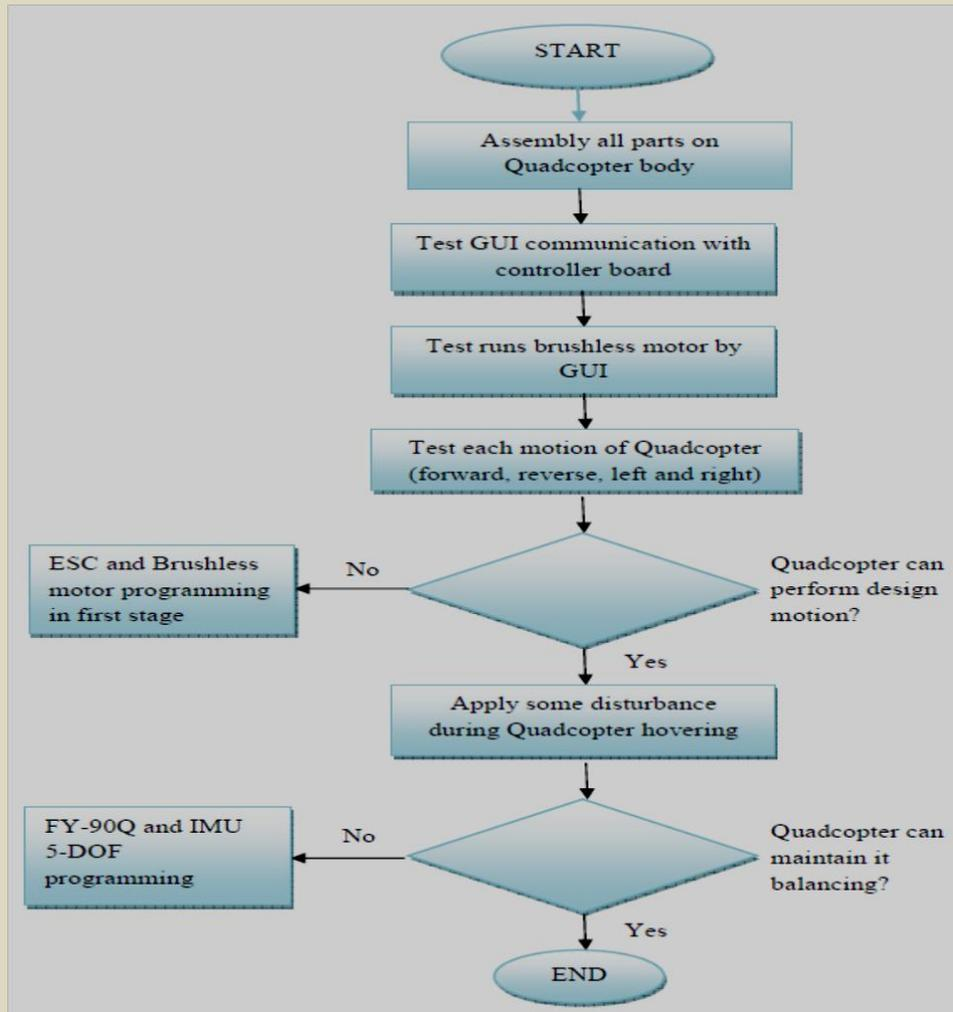
Figure 3: Flow chart of quad-copter design
