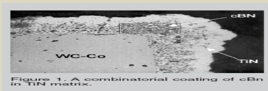
Figure 1. A combinatorial coating of cBn in TiN matrix.
